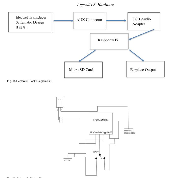
Fig. 19. Schematic Design [8]
